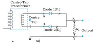
Principle:- Diode conducts only in forward biasing. Input D<sub>1</sub>
